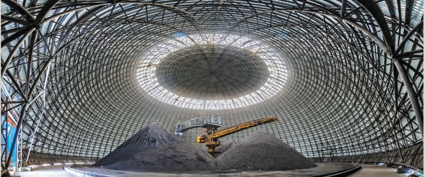
Interior view of the stacker reclaimer of the coal washery at Satna.
