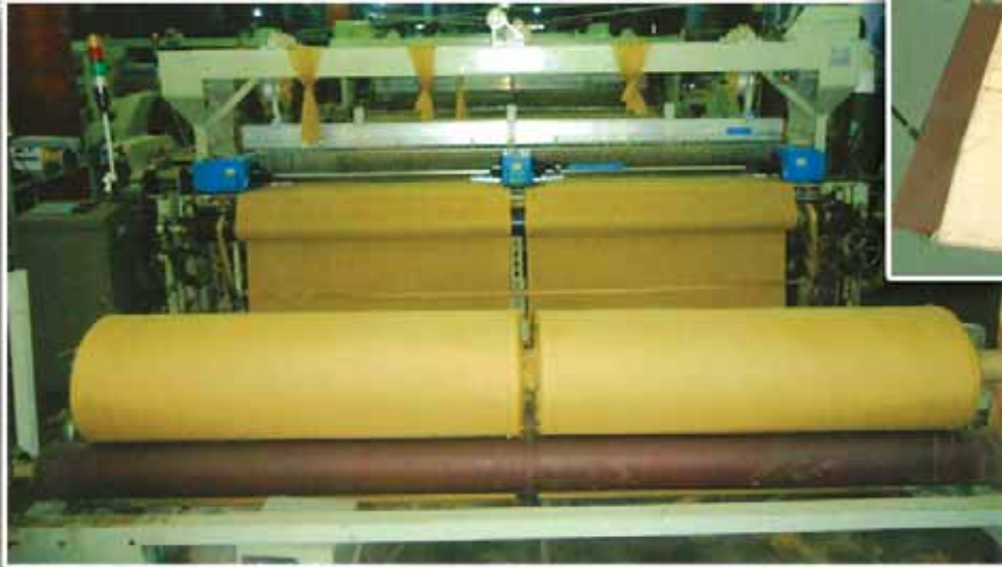
The modern shuttleless flexible Rapier Victor loom at Birla Jute Mills, Birlapur, West Bengal; (inset) the Flexographic printing machine
