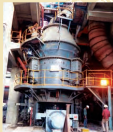
Vertical roller mill for pet coke grinding at Satna.
