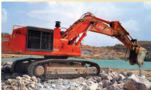
Mechanical mining of limestone at Jai Surjana Mines, Chanderia.
