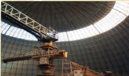
Inner view of the new limestone stacker & reclaimer at Chanderia.
