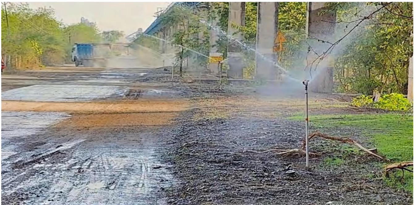
Fixed Water Sprinklers along Haul road
