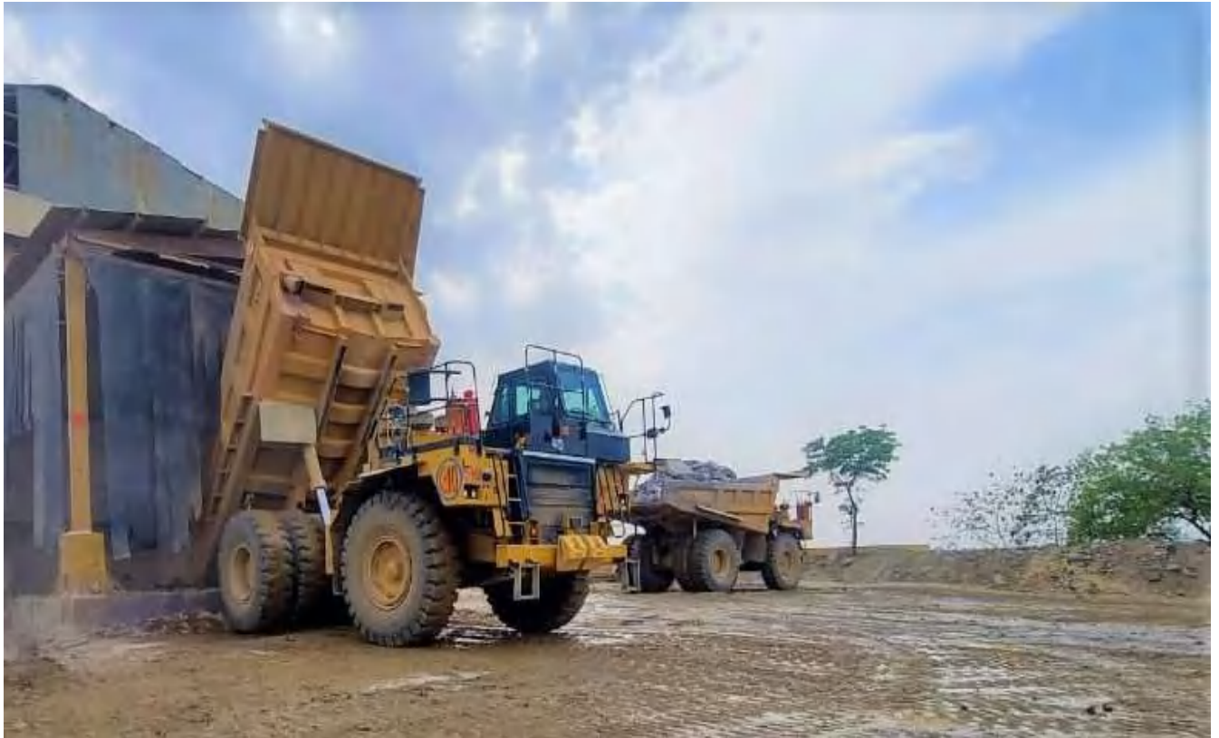
Covered hopper to control fugitive emission
