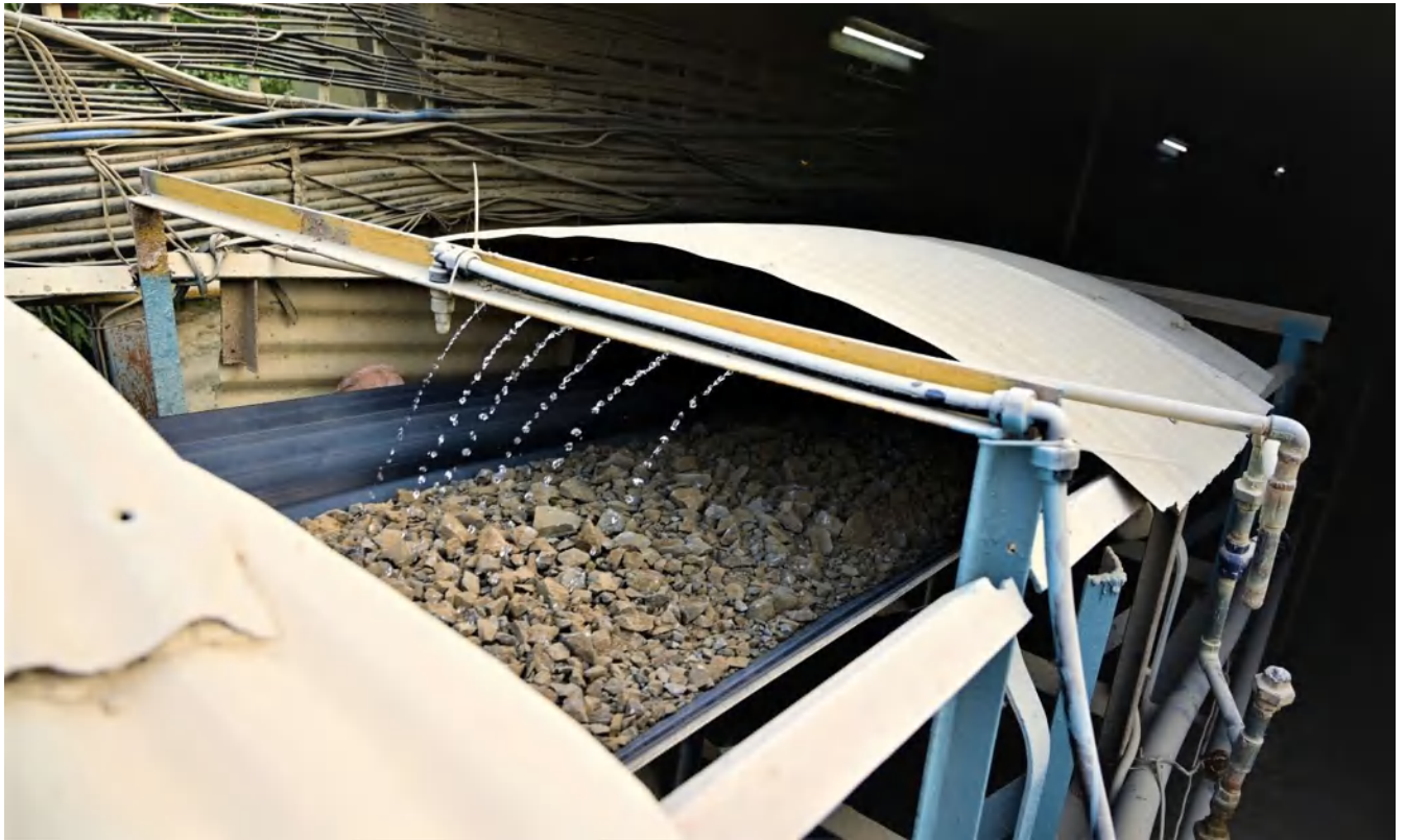
Water spray system installed at conveyor belt
