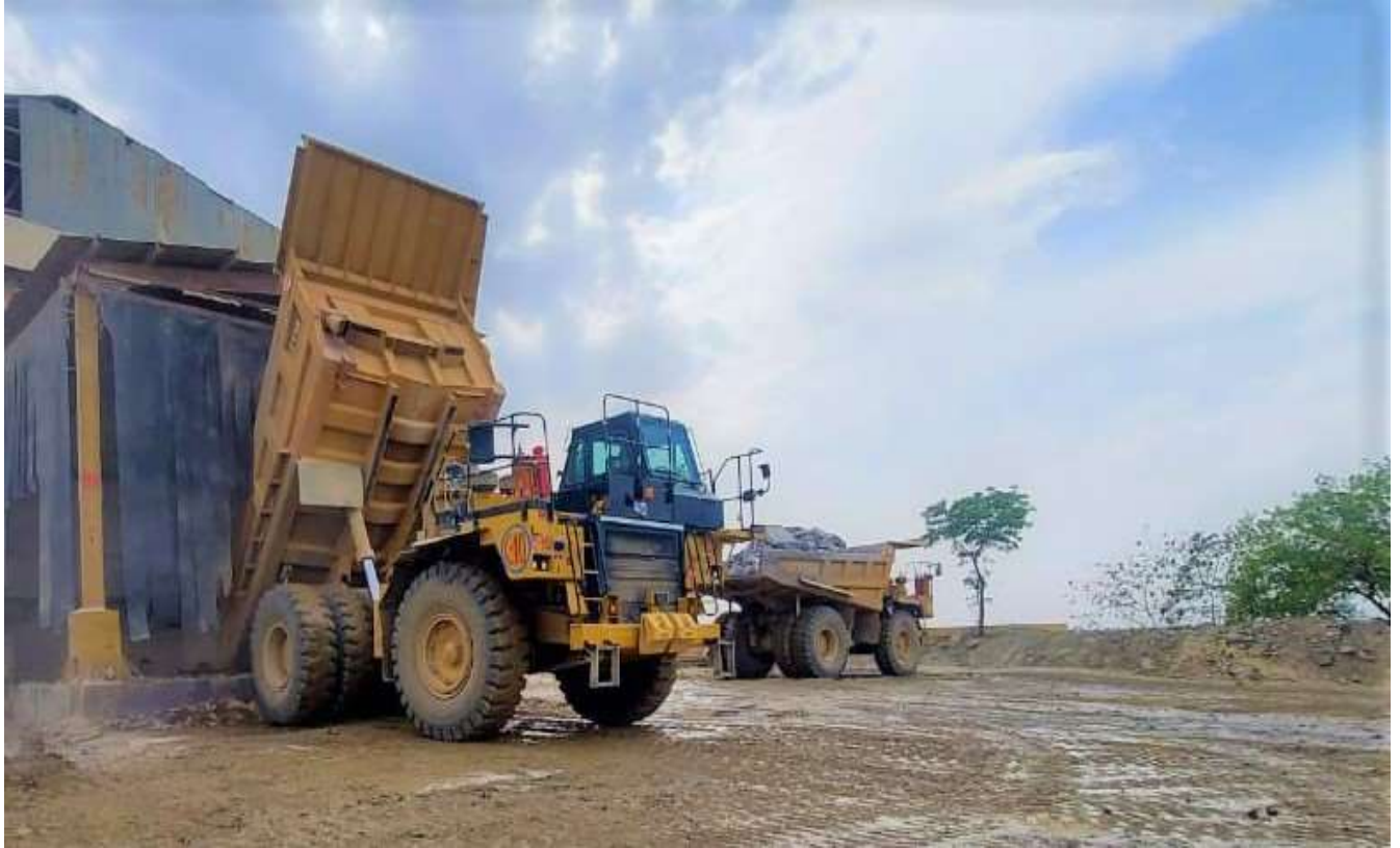
Covered hopper to control fugitive emission
